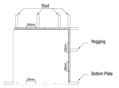
Establish a horizontal datum line where, as a minimum, the bottom edge of the sheet overhangs the bottom plate by 20mm. Plan sheet layout with the rebated faces either:
