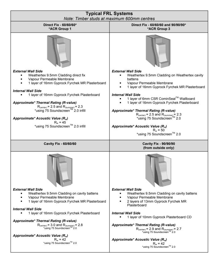
Note: The timber framed and steel framed FRL systems in this guide are indicative of typical systems provided by CSR Gyprok. Application must be in accordance with the system manufacturer's installation requirements and instructions.
