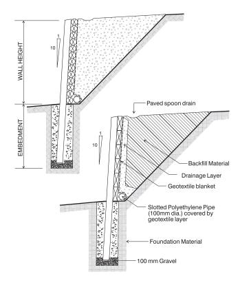
Figure 2 - Log and sleeper retaining walls
