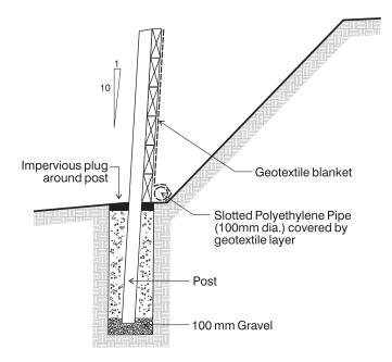
Figure 6 - Wall prior to backfilling
