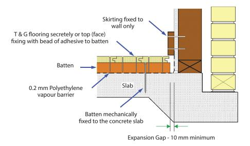
Figure 4 - Fixing to battens
