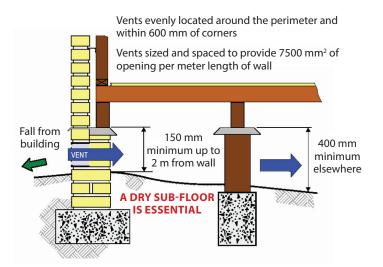
Figure 1 - Sub-floor Ventilation
