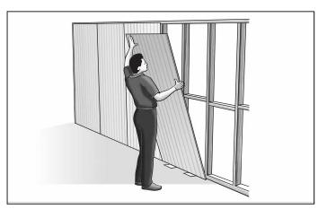
**FIGURE 4 SHEET INSTALLATION**
