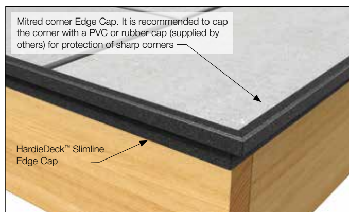
FIGURE 10 EDGE CAPPING MITRED CORNER DETAIL
