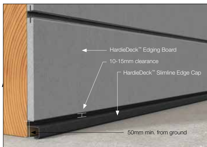
FIGURE 12 BOTTOM FINISHING DETAIL AND CLEARANCE
