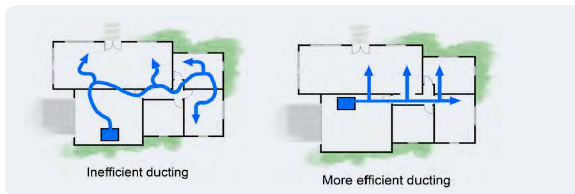
Figure 71: Duct runs. Straight duct runs improve efficiency.
