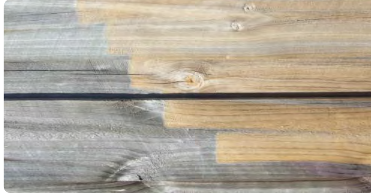
Figure 9: Weathered, grey surface adjacent to unweathered surface.
