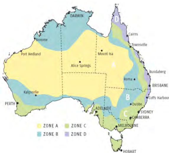
Figure 13: Above-ground decay hazard zones. (Zone D has the highest decay potential.) Source: Wood Solutions Guide #5 Timber service life design guide
