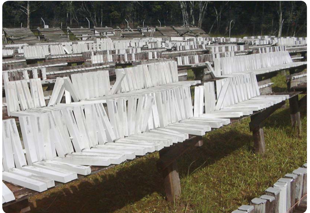
Above-ground durability test site in South-East Queensland.
