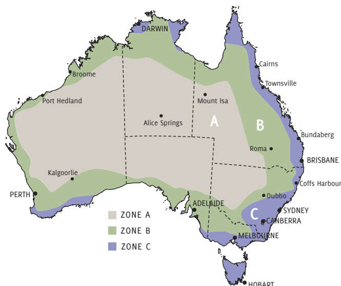
Figure 5: Hazard zones for embedded corrosion. Zone C has the highest hazard.
